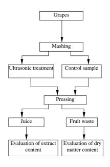
Fig. 1. Flow diagram of juice grape pressing
