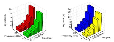
**Fig. 5.** Dry matter content as a function of frequency and time of sonication for grape variety Portugalskie Niebieskie
